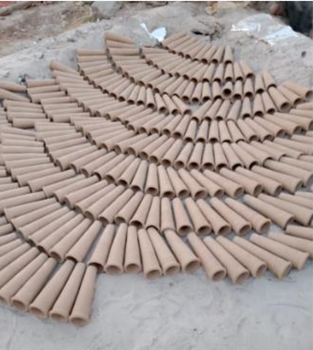
Drying & Firing of terracotta pipes at pottery
